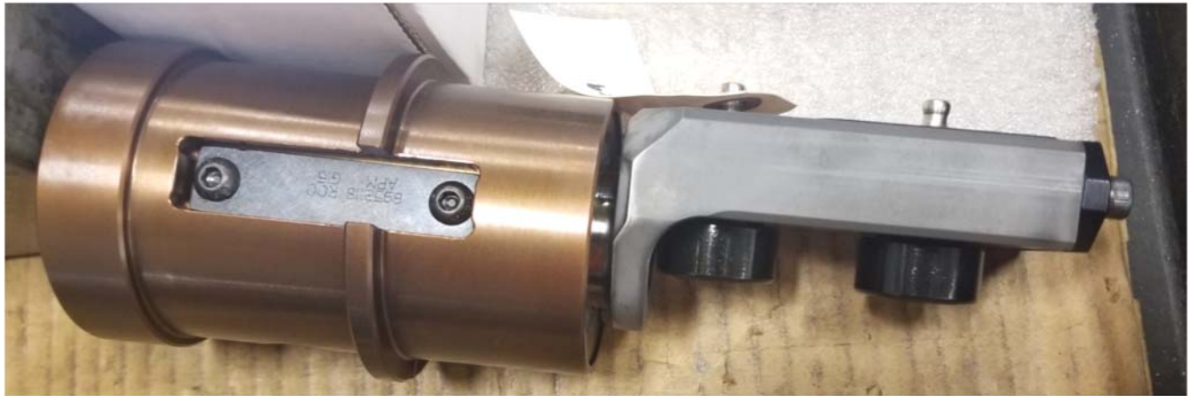
Cam Followers installed on The Belvac and Servo Belvac style ram assembly
