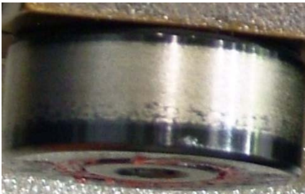
Figure 6: Significant wear on the surface of the Cam Follower. It is recommended to replace the part.
