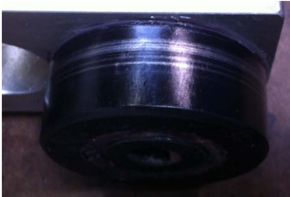
Figure 5: Light wear on the surface of the Cam Follower. It is common to see wear of this magnitude after the first full day of running the machine.
